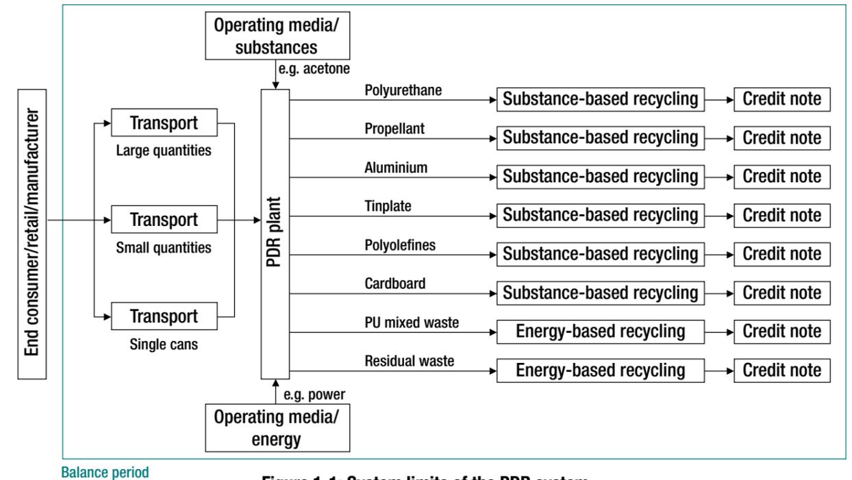
Figure 1-1: System limits of the PDR system
